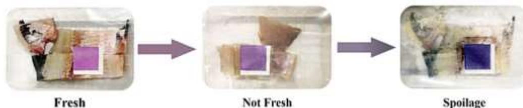
Fig 3. Changes in paper sensors' colour indicating grass carp freshness within 24 h at 25 °C (Sun et al, 2021).
